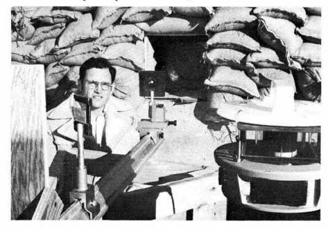
BOB BENHAM (1533) test engineer, uses a laser beam to position the fuze target in front of the explosive barrel and flyer plate at the Thunderwell facility south of Area III. Precisely controlled impact angles and velocities are achieved with the new testing technique.
